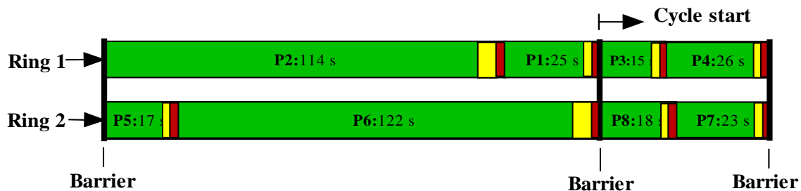
Figure 2.3: Dual-ring control diagram of intersection TH 55 & Boone Ave during weekday AM peaks.
