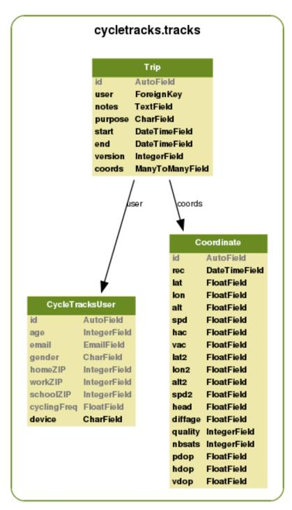
Figure 2.2: UMN CycleTracks back end server database model.
