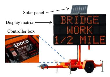
Figure 2.1: PCMS used in the research project.
