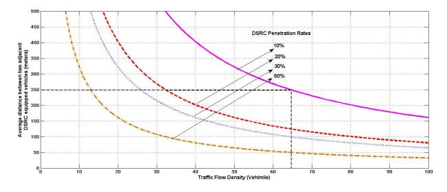
Figure 5.2: Average distance between two adjacent DSRC-Equipped vehicles as a function of traffic flow density for different DSRC penetration rates.
