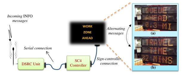
Figure 4.2: Snapshots of the PCMS display matrix showing alternate messages of (a) distance to the queue ahead and (b) travel time.
