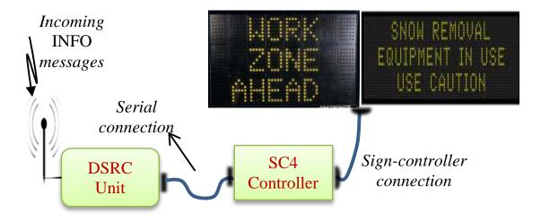
Figure 2.2: Schematic diagram of DSRC-PCMS hardware interface.
