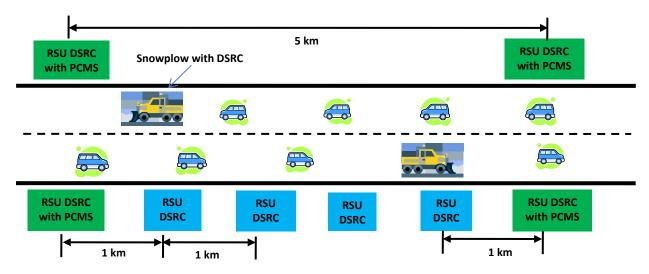
Figure 3.1: The schematic diagram of Snowplow Warning System using V2I and/or V2V based DSRC communication and PCMSs.
