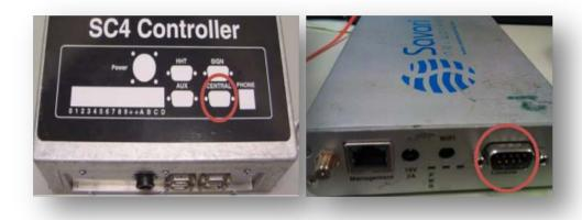
Figure 2.3: (a) Top view of the SC4 controller deluxe version, and (b) Serial console of Savari DSRC unit.
