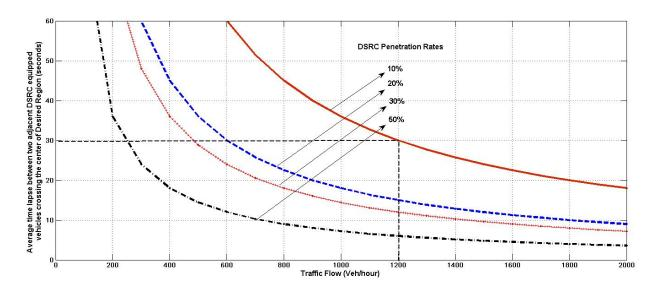
Figure 5.1: Average time lapse between two adjacent DSRC-Equipped vehicles crossing the center of the *Desired Region* as a function of traffic flow for different DSRC penetration rates.
