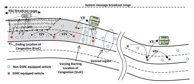
Figure 4.1: Conceptual architectural diagram of the developed hybrid DSRC-PCMS information system for work zone.
