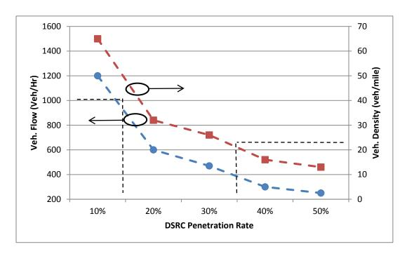
Figure 5.3: Required traffic flow and density for a given DSRC penetration rate.
