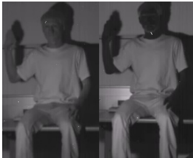
Figure 1. A pair of images taken by the infrared cameras is shown. The left image captures the wavelengths from 900 nm to 1400 nm, while the right image is from 1400 nm to 1700 nm. Most objects appear similar in the two images, while skin is significantly less reflective in the higher wavelengths.
