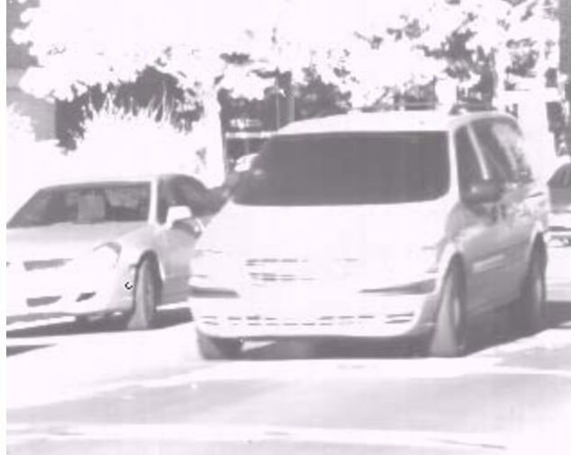
Figure 10. Infrared reflective glass prevents the majority of infrared illumination from entering a vehicle. Currently this technology is uncommon in the United States, but may increase in the future due to its energy savings.
