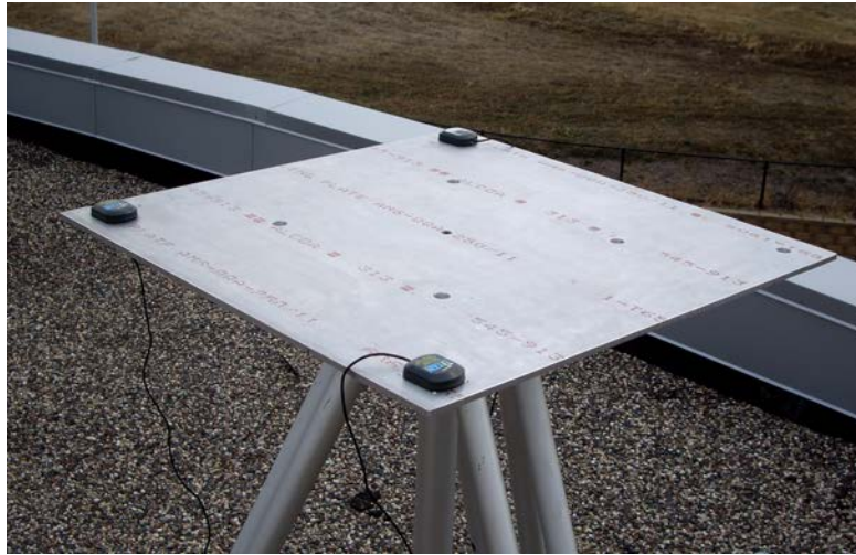
Figure 3.6: Phase center calibration test setup
