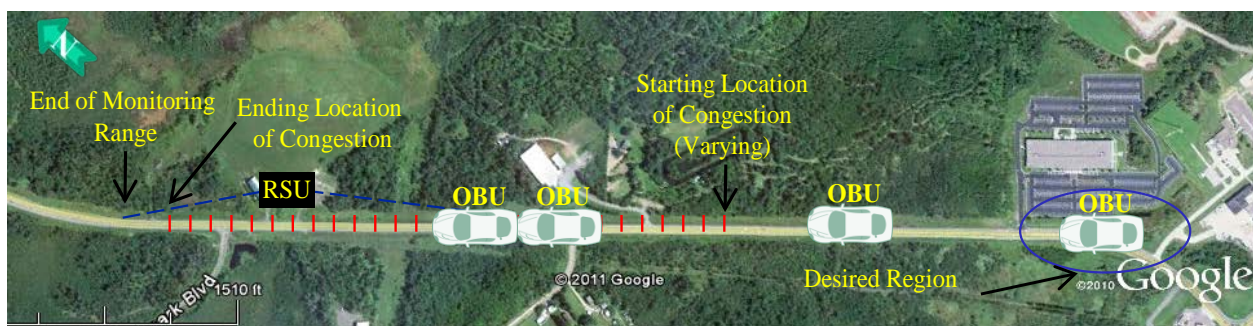
Figure 4-2: The Field Demonstration Site Showing Placement of DSRC Units and the Coverage Range of V2V-Assisted VI Traffic System.
