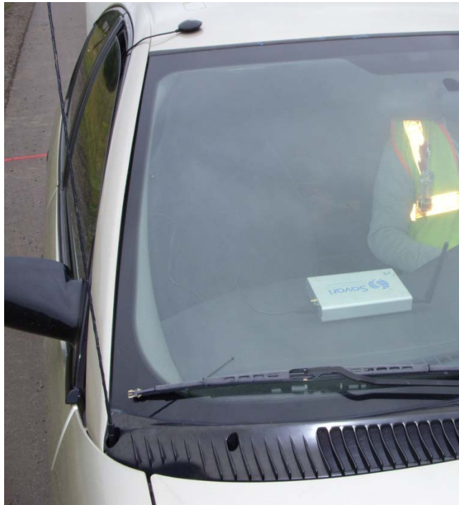
Figure 4-1: The Placement of the OBU in Test Drive Vehicle
